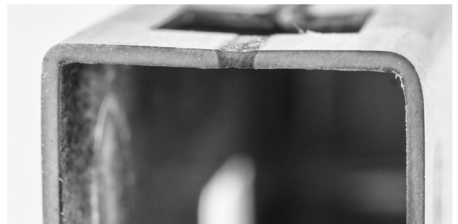
Example of laser welded steel profile.
